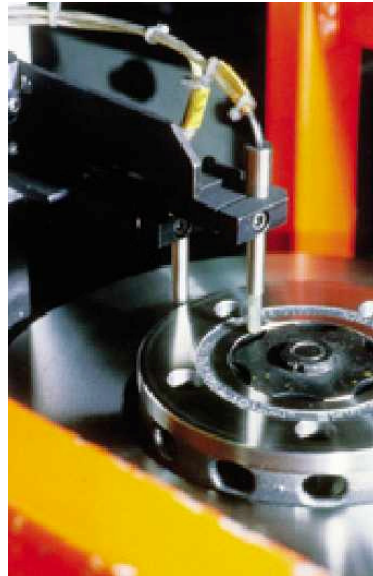
Fig. 2: Probe pusher puller unit with two probes
